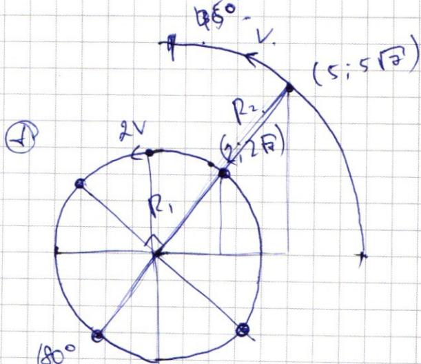
$$\alpha' = \frac{2Vt}{2\pi R_1} = \frac{Vt}{\pi R_1} ; \quad \alpha'' = \frac{Vt}{2\pi R_2}.$$
