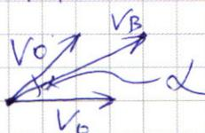
$$v_B = \sqrt{(v_0 \cdot \sin \alpha)^2 + (v_0 \cdot \cos \alpha + v_0)^2} =$$
