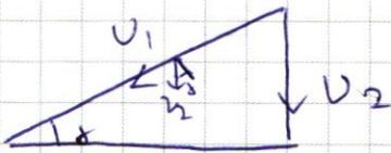
$$\sin \alpha = \frac{v_2}{v_1}$$
